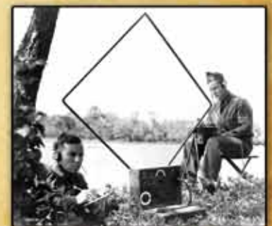
Signal Corps Soldiers, in the 1930s, operating a superheterodyne radio receiver, which amplified weak signals and enabled more precise tuning
