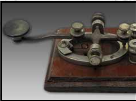
U.S. Army wired telegraph key patented circa 1881
