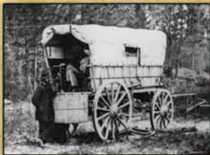
Trains - or more specifically, light wagons - were used to carry telegraph sets and other necessary items, such as reels of insulated copper wire and iron lances, for stringing temporary field lines, called "flying telegraph lines".
