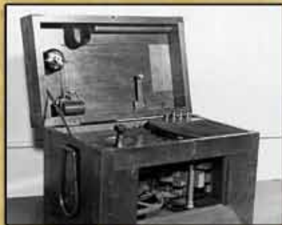
The magneto-electric telegraph, invented by George W. Beardslee generated current by turning a set of cranks to revolve magnets. The Signal Corps employed this machine because it did not require operators trained in Morse code.
